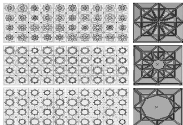
Figure 5. CABS system opening ratios ranging from 10% to 90%
