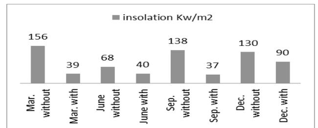
Figure 11. Solar Irradiation with and without CABS
