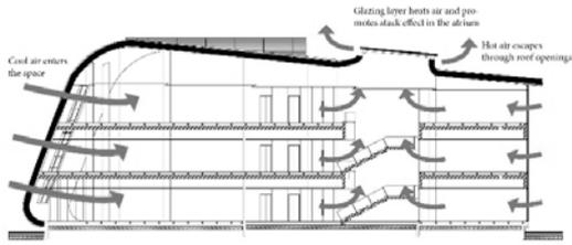
Figure 17. Stack effect ventilation
